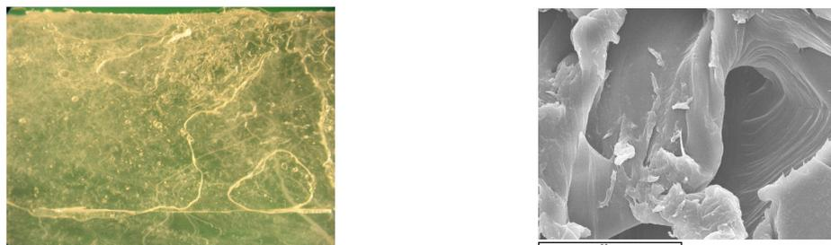
**Figure 3.** Morphology of rough typology ultimate shear, a) macro-8x, b) SEM micrograph at 2000 magnification.
